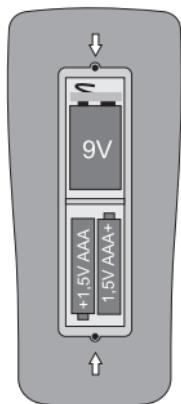
Do not leave flat batteries in the device. Even batteries protected against leaking can corrode and thus release chemicals which may be detrimental to your health or destroy the device.
