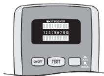
You can use the cable tester to check that network lines are functioning and connected correctly (note the appropriate pin assignment for the different wiring systems).
