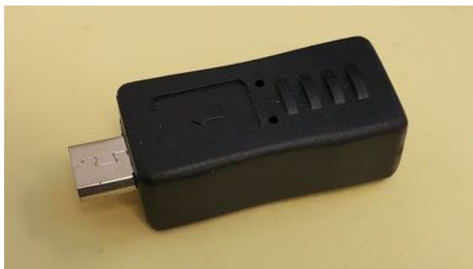
Figure 17: Android Connector Reverser #1
