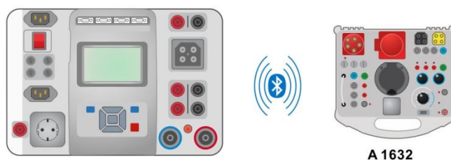
Figure 8.4: Connection of the eMobility Analyser (A 1632)
