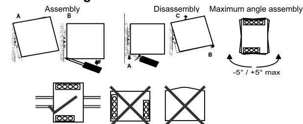
**Other models / modules** must have a minimum vertical and horizontal distance of 10 cm to this power supply in order to guarantee sufficient auto convection. Depending on the ambient temperature and load of the device, the temperature of the housing can become very high!
