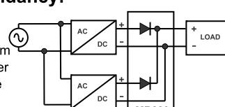
This can be done by utilizing decoupling
