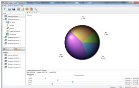
The analyzer has four independent Measurement Points. Each Measurement Point can be set individually to perform four different types of registration without need to change analyzer's configuration.
